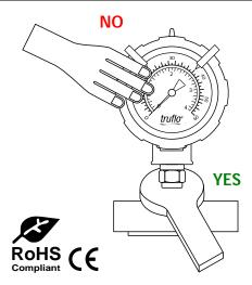
After installation the vent plug can be cut to relieve internal pressure changes in the gauge case that otherwise would have been induced by environmental changes in pressure and/or temperature. Without being vented this change in internal pressure could adversely affect the accuracy of the gauge. If liquid filled, only open vent plugs when the plug is oriented in the vertical position.
